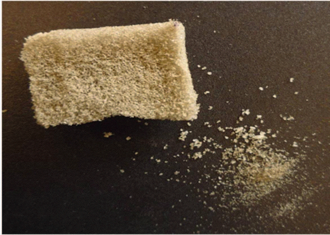
Figure 30. PUR ether foam crumbled after ageing treatment by UV radiation
