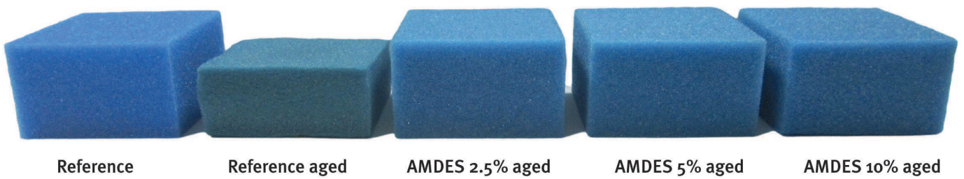
Figure 39. Macro images of untreated and treated samples after compression test (5 x 5 x 3 cm)
