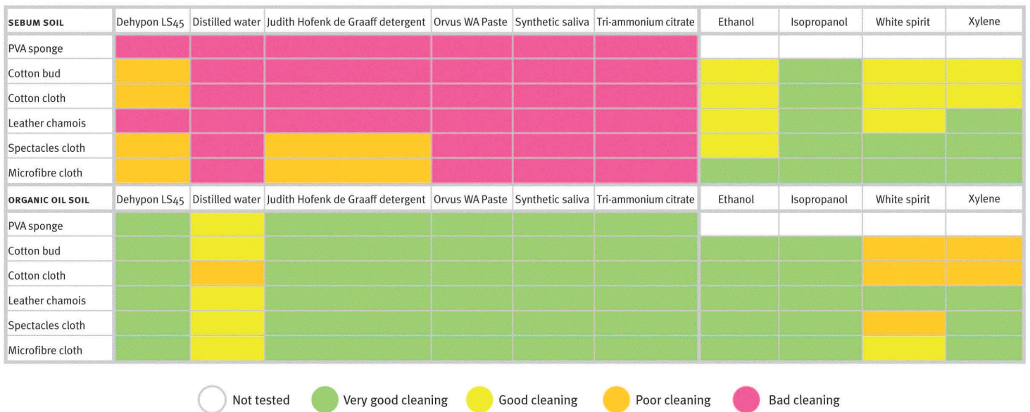
Figure 4. Visual examination of soiled CA after cleaning
