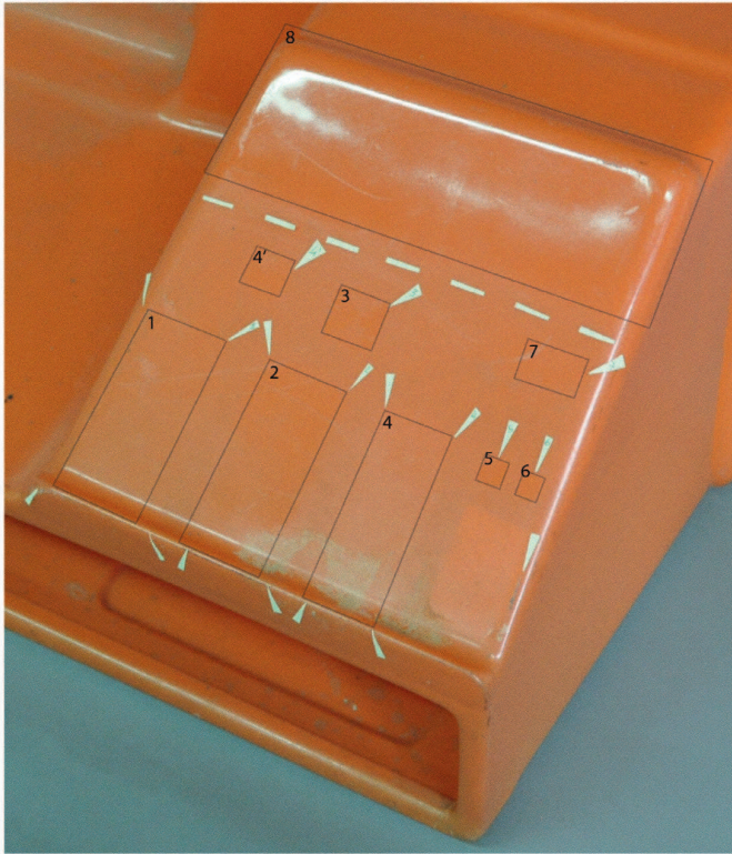
Figure 21. Detailed photograph of wall storage furniture by Jean-François Lecoïnte showing cleaning: 1. Microfibre cloth/ Orvus WA Paste, 2. Microfibre cloth/ Dehypon LS45, 3. Cotton bud/ Dehypon LS45, 4. Spectacles cloth/ tri-ammonium citrate, 4'. Cotton bud/ tri-ammonium citrate, 5. Cotton bud/ ethanol, 6. Cotton bud/ isopropanol, 7. Spectacles cloth/ ethanol, 8. Large area cleaned with cotton bud/ethanol (© Clémentine Bollard)
