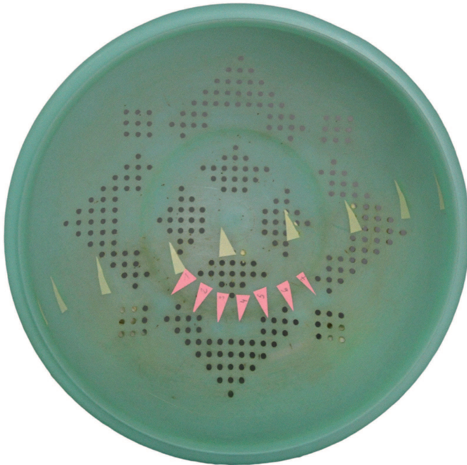
Figure 20. Tupperware polyethylene strainer, upper side after cleaning and lower part showing test areas: 1. Cotton cloth/ tri-ammonium citrate, 2. Microfibre cloth/ Orvus WA Paste, 3. Microfibre cloth/ Judith Hofenk de Graaff detergent, 4. Microfibre cloth/ distilled water, 5. Cotton cloth/ Dehypon LS45, 6. Cotton bud/ isopropanol, 7. Cotton bud/ ethanol (© Clémentine Bollard)
