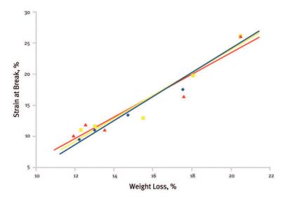
Figure a. Percentage weight loss versus the strain at break for the samples aged at 70°C and 30%, 50% and 70% RH. Tensile tests carried out using a 500 N load cell, gauge length of 50mm and a crosshead speed of 5 mm.min<sup>-1</sup>. Thermogravimetric analysis on samples weighing in the region of 5mg over a temperature range of 30 to 450°C at a heating rate of 5°C.min<sup>-1</sup>
