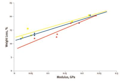
Figure b. Difference in flexural modulus between 5 minutes and 120 minutes versus percentage weight loss for the samples aged at 70°C and 30%, 50% and 70% RH. Dynamic mechanical analysis carried out using a three-point bend at constant temperature of 24°C, performed over a period of 120 minutes at a frequency of 1.0 Hz. Thermogravimetric analysis on samples weighing in the region of 5mg over a temperature range of 30 to 450°C at a heating rate of 5°C.min<sup>-1</sup>
