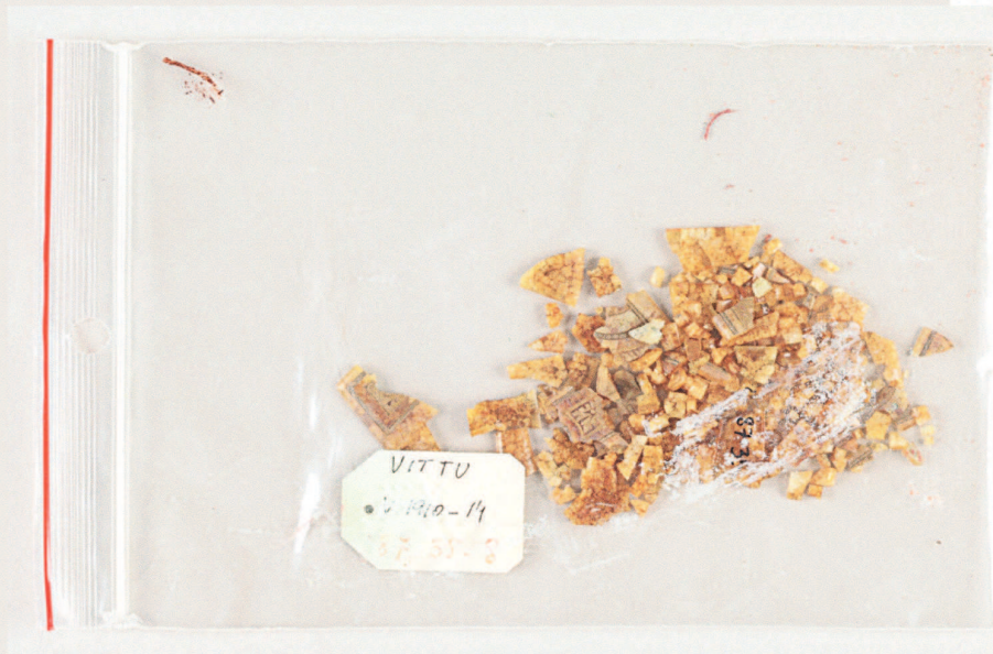
Figure 1. Comb, ca. 1910 example of a celluloid object (Cellulose nitrate plasticised with camphor) at its final step of degradation (© C2RMF, photo Thomas Clot)
