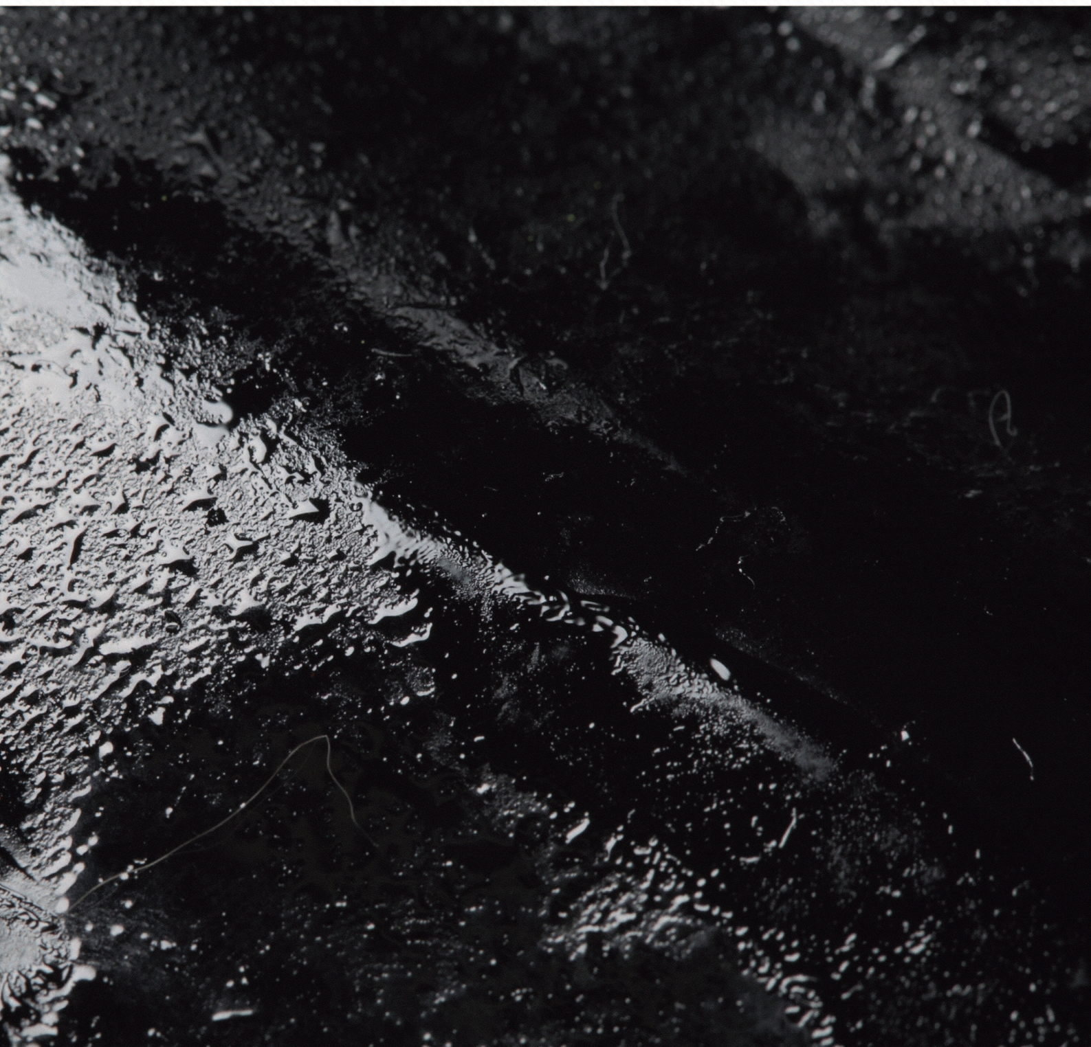
Figure 2. Paco Rabanne: Raincoat (detail). Drops of phthalate plasticisers on the surface of the PVC (© C2RMF, photo Thomas Clot)
