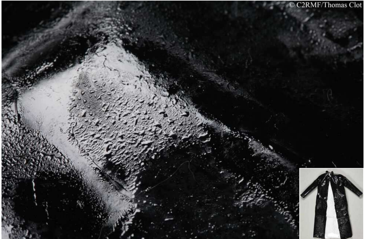
B- Raincoat (1978) : - sweating of phtalates plasticizers in the form of drop - sticky surface
