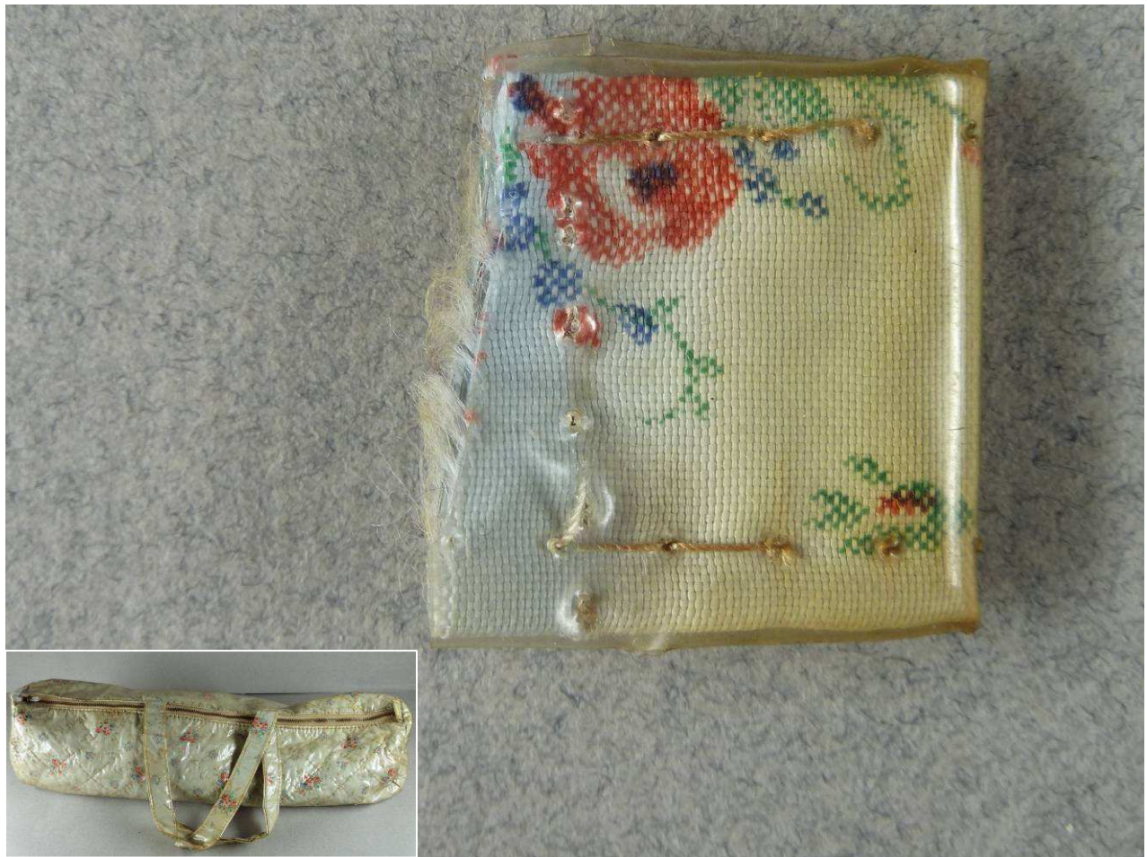
C – Purse handle, embroidery covered with a PPVC sheet : yellowing © RCF
