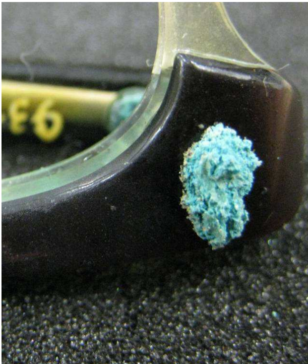
H- Glasses : Corrosion of metallic element (copper alloy) © C2RMF
