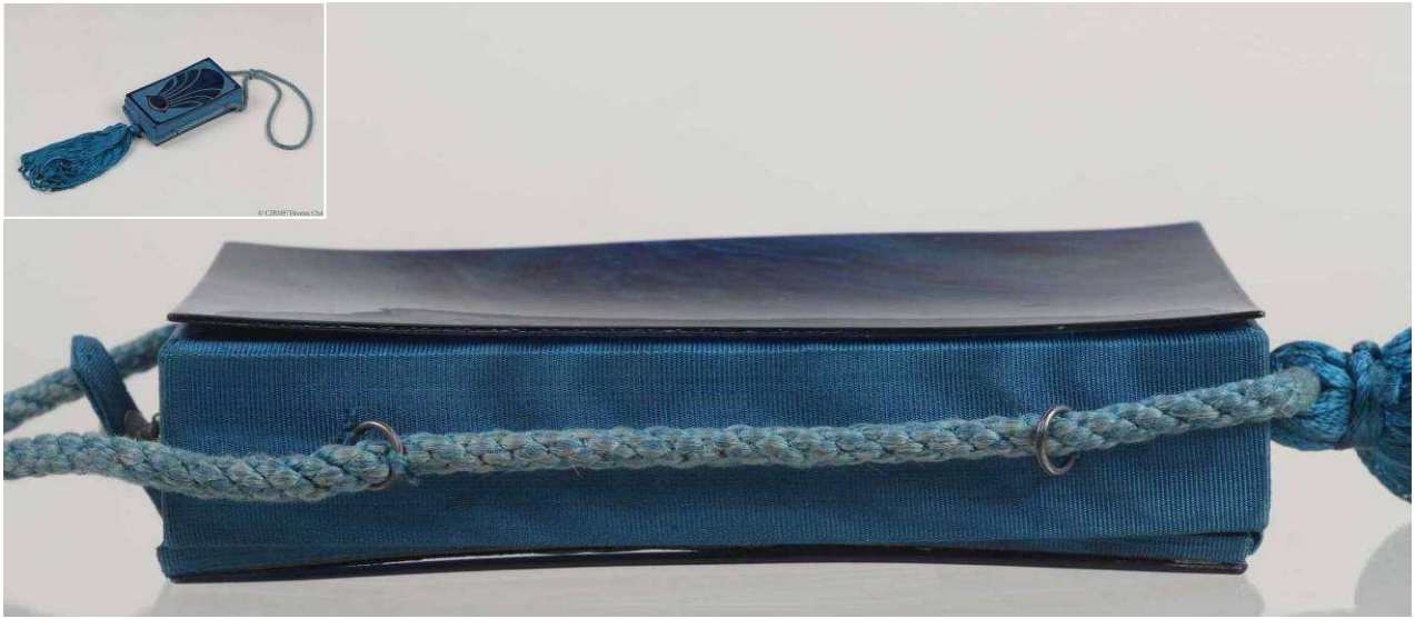
A – Purse (1920s) : warping , shrinkage © C2RMF
