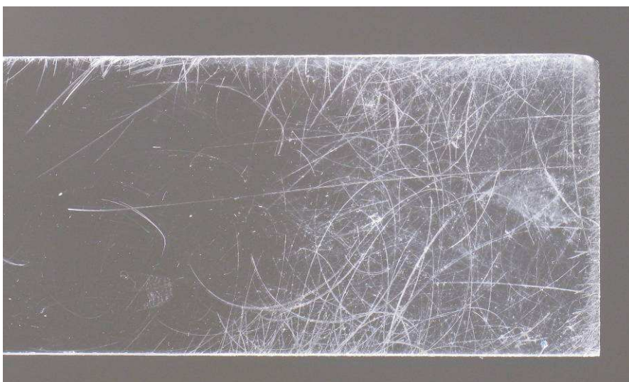
C- Transparent plate : Scratch and abrasion , causing a loss of transparency and change in gloss - © C2RMF
