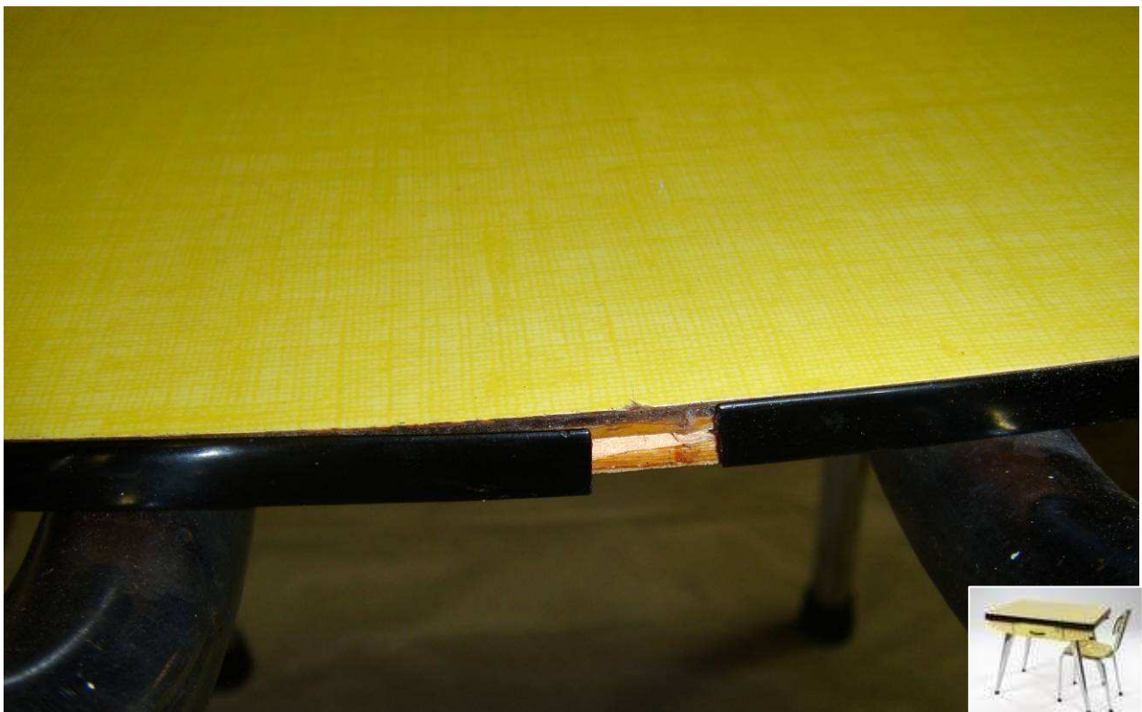
D- Chair, metal, melamine formaldehyde resin (Formica®) and PVC (1960) : shrinkage of the black PVC strip (© C2RMF)
