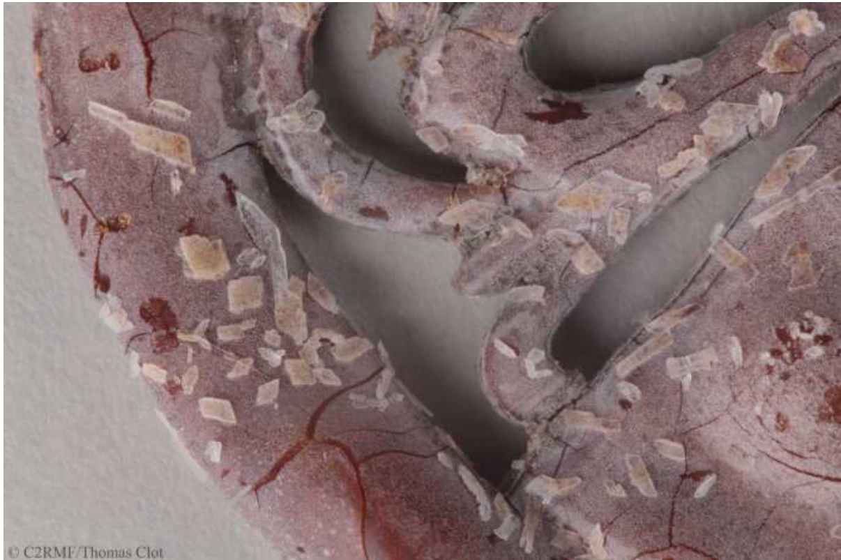
C – Comb : bloom (solid deposit made of exuded and dried plasticizer) associated with loss of transparency, change in gloss and crack © C2RMF
