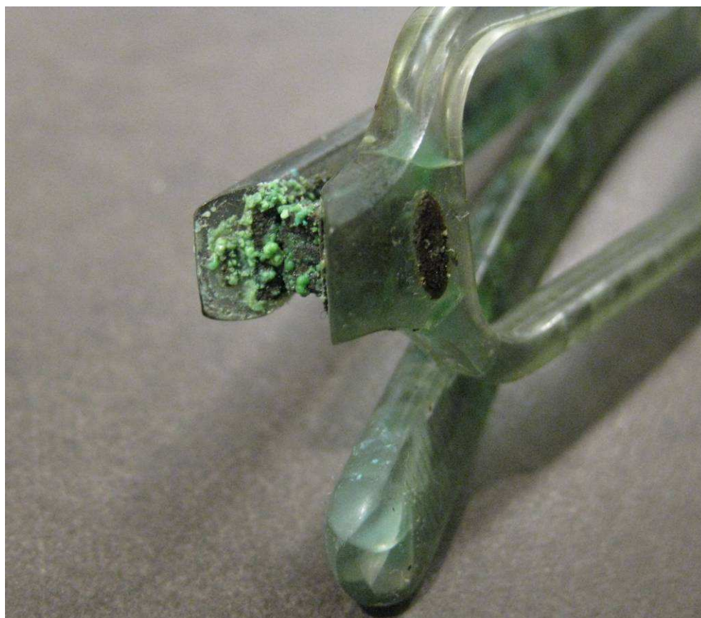
E - Glasses : corrosion of metallic elements © C2RMF
