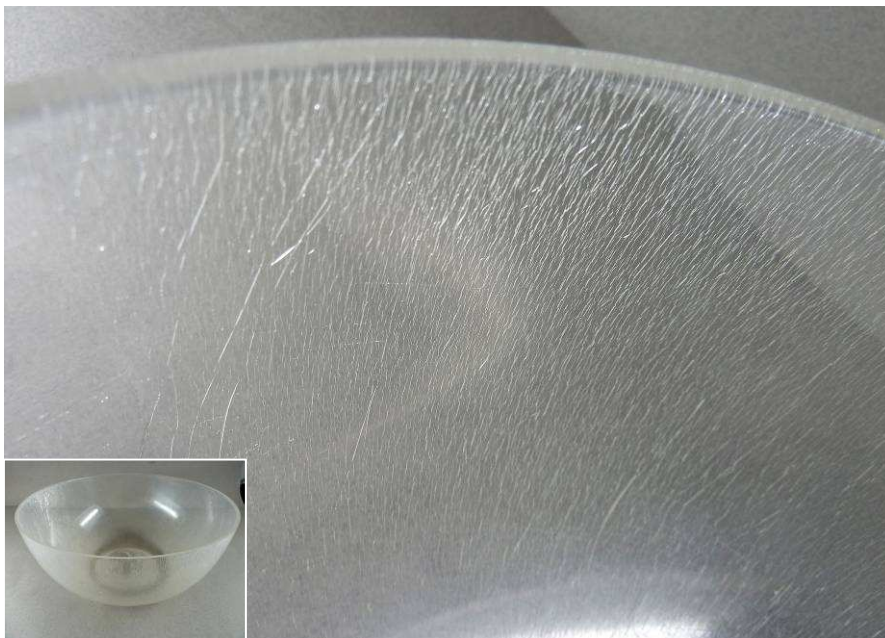
B- Salad bowl : crazing , causing a loss of transparency - © RCE
