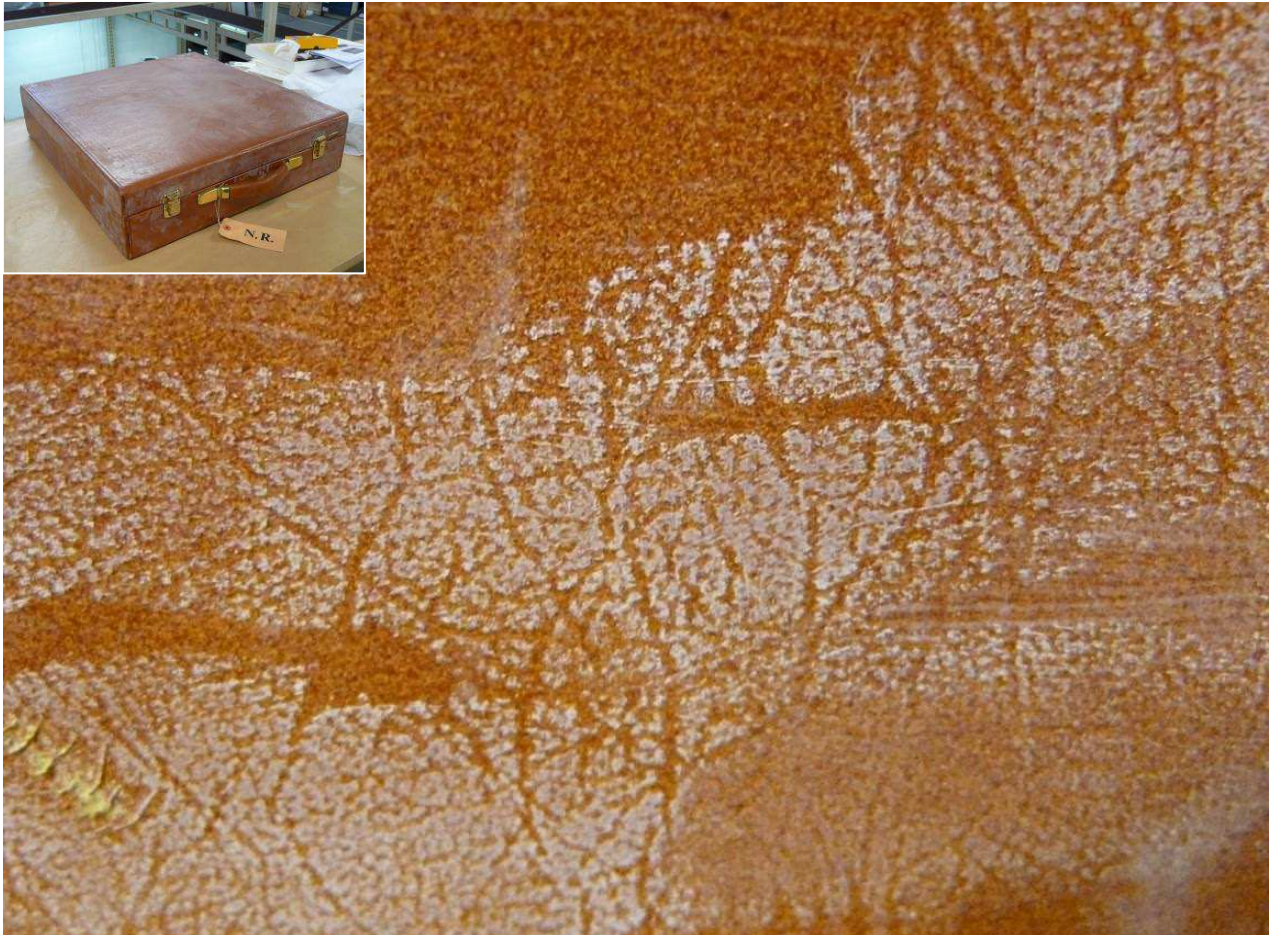
3 - Suitcase coated with leatherette (1960s) : bloom (unzipped polymers of PUR ester) © C2RMF
