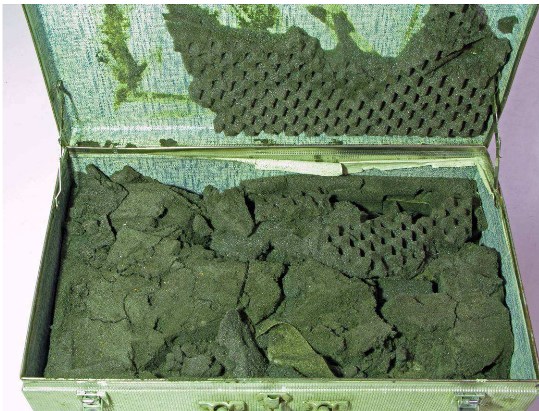
B – suitcase cushioning (1970s): PUR ester foam become brittle and crumbly © C2RMF
