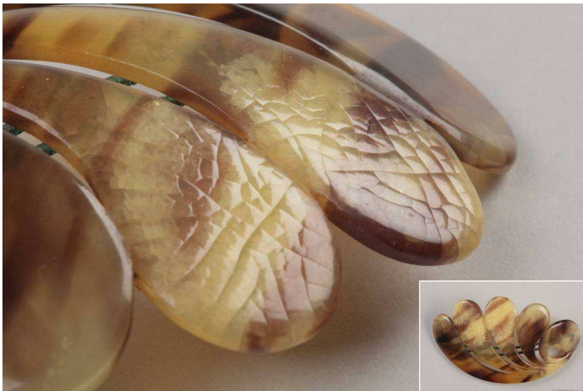
A – Hair slide, tortoiseshell imitation : crazing , associated damage : loss of transparency © C2RMF
