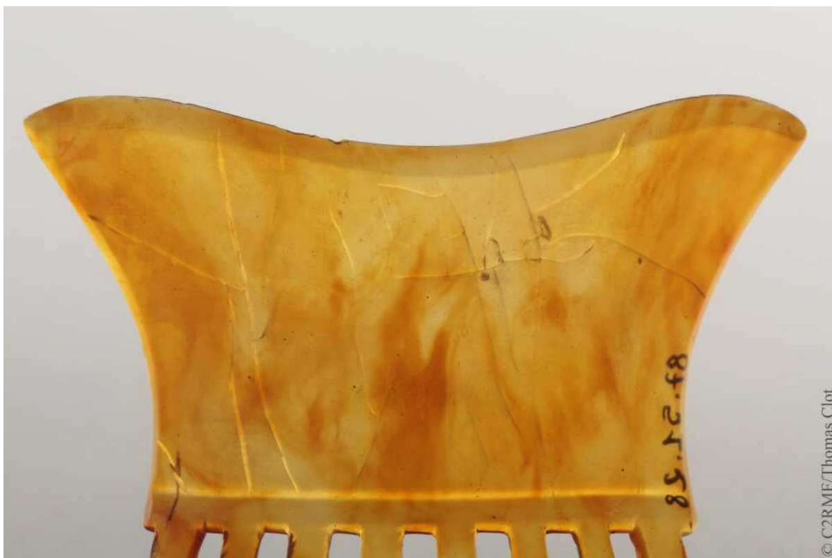
B – Comb (horn imitation): crack © C2RMF
